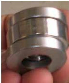
Figure 3.10 Load Cell used to measure prestressing force
