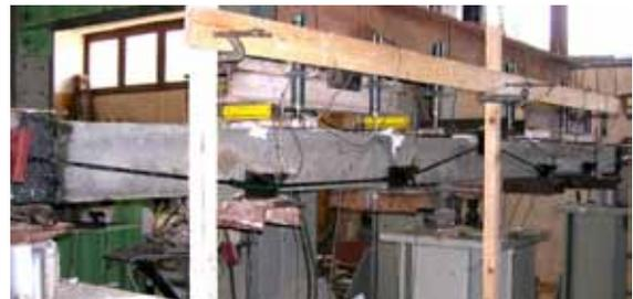
Figure 3.12 Arrangements of LVDT's for deflection measurements (back view)
