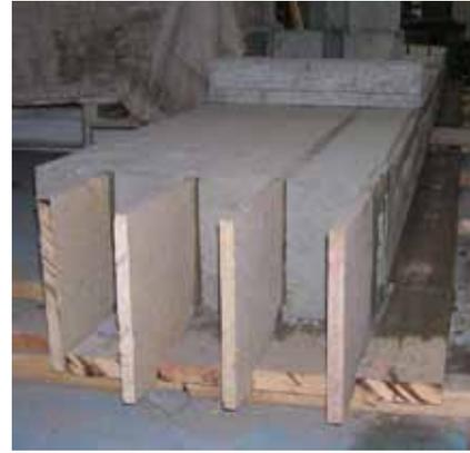
**Figure 3.4** Mould of test beams
