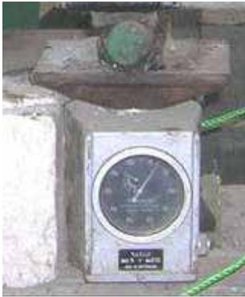
Figure 3.13 Load cells at external supports
