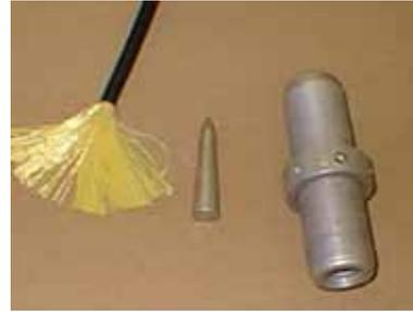
Figure 2.14 Parafil rope and its anchorage and Installation procedure for Parafil rope
